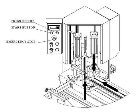
10.8. Press the start button to remove the gauge. Pull the movable head until the profile sticks to the gauge.
